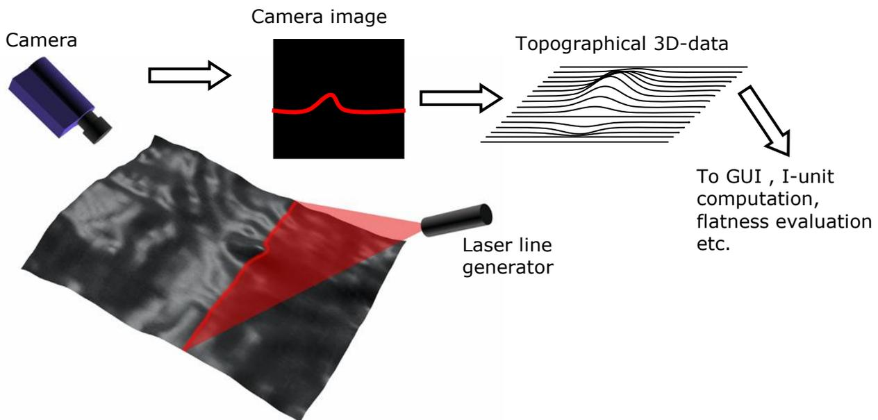
Figure 1. The principle of laser line triangulation
