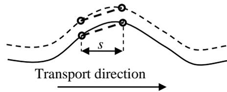
In each width position, two points are measured giving a local slope or gradient. Even if there is a vibration, the gradient is the same.
