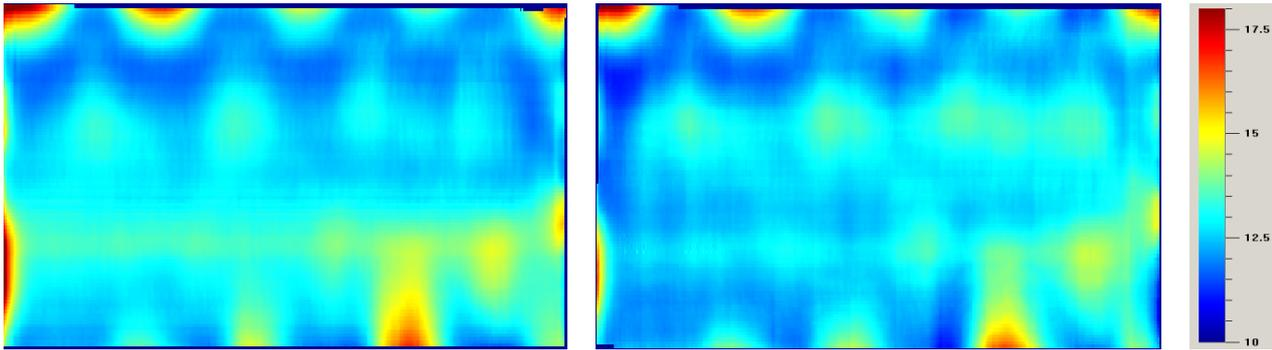
*The same plate measured on a stone table (left picture) and on a roller table (right picture)*
