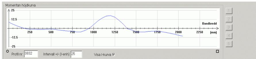
I-unit profile. Computed from the topography. Used for quality assurance, leveller control or mill control.
