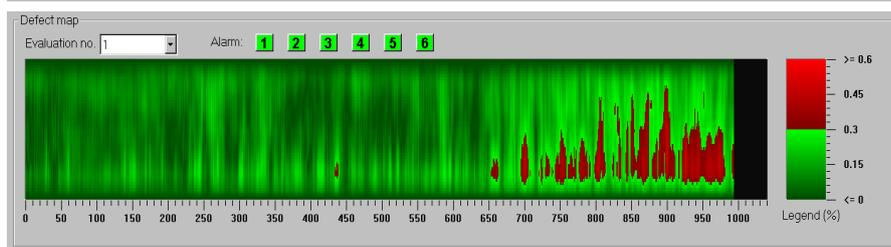
Defect map. Shows which parts that do not fulfil the end-customer requirements.
