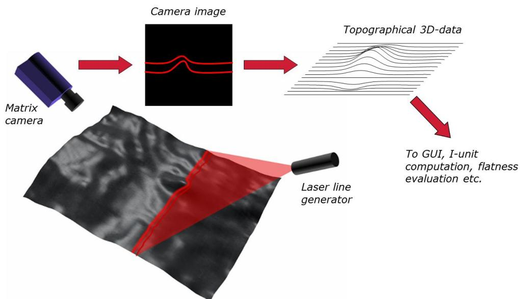
Figure 1. The principle of laser line triangulation
