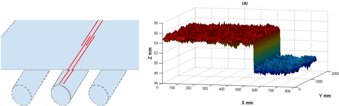
Figure 3. The strip and a supporting roll were measured at the same time (left), which resulted in two different surfaces influenced by heat-shimmering (right).
