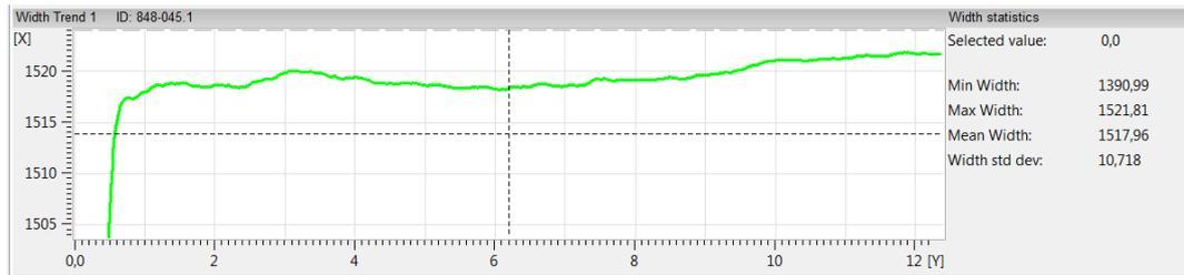
Figure 13. Strip width graph from a strip head
