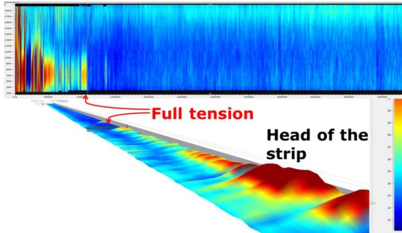
Figure 10. An example measurement. The top graph shows color coded topography for the major part of the strip. Underneath is a 3D-graph of the same data seen from strip head position.
