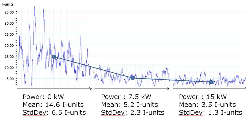
Figure 6. I-units introduced by heat-shimmering. Three different measurements were done on the same coil with a change of fan power between the measurements.
