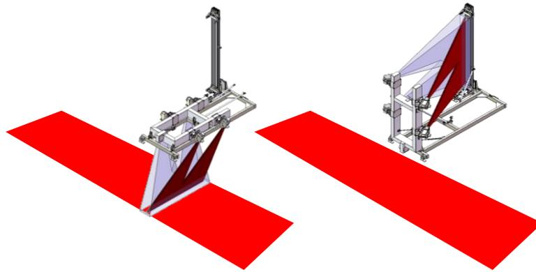
Figure 8. Schematic arrangement of the measurement system. The left figure shows measurement position and the right shows calibration position.
