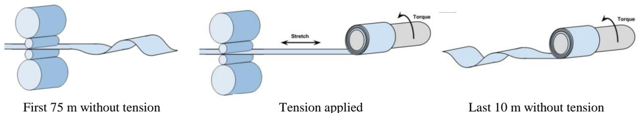
Figure 9. The three rolling phases.
