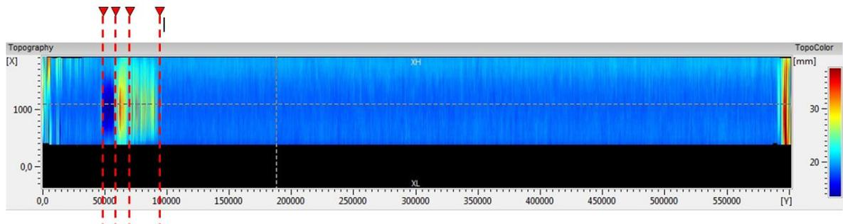
Figure 14. A strip where the mill-stand changes Triangles indicate where the rolling mill parameters were changed.
