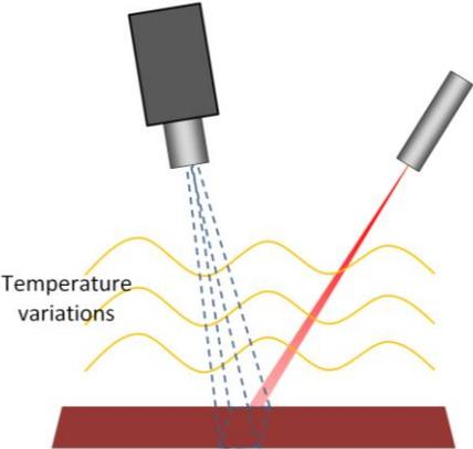
Figure 2. Air temperature variations cause the light rays to “bend” which results in optical distortions in the camera pictures.
