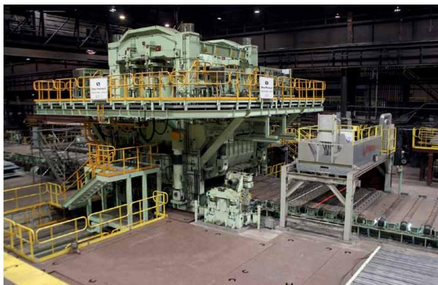
Figure 1. New 4-m wide plate leveller at ArcelorMittal Burns Harbor works (Courtesy: ArcelorMittal)
